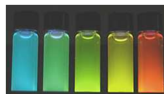
Figure 2: Brightly glowing water soluble CdSe/ZnS nanocrystals
