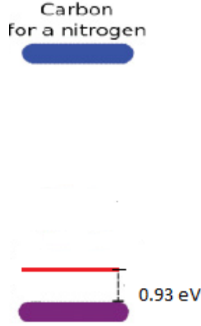
FIGURE 14 – The level of the defect in red, the valence band in violet and the conduction band in blue.
